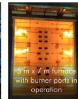
5 m x 7 m furnace with installed test specimen
